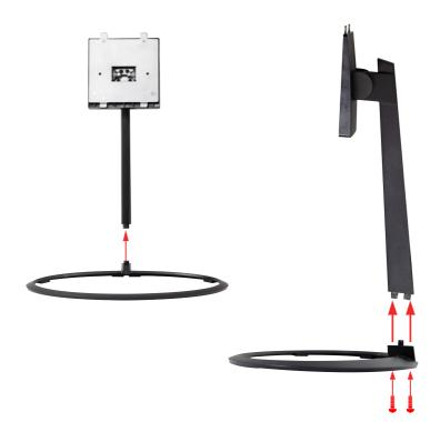
2. Insert the neck into mounting hole , then press down until you hear the locking clip lock down.
