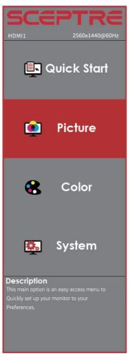
When you press the 0 button on the monitor, the OSD screen will appear. Select each of the functions with the joystick  $\blacktriangle$  or  $\blacktriangledown$ . Use the 0 button again to enter each of the function or when you are in the function already, use the 0 button to select the option you want to adjust. Use the joystick  $\bigstar$  or  $\blacktriangledown$  to adjust each option's values. When you want to exit push the joystick leftwards.
